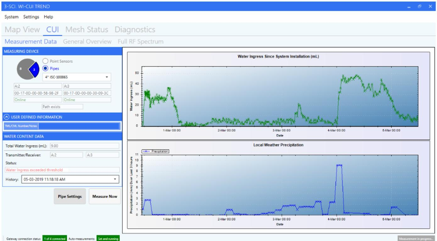
Wi-Corr user interface demonstrating a correlation between detected water ingress inside the cladding and local rainfall
