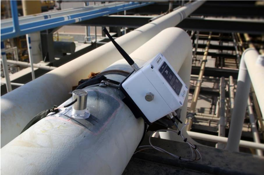
Wi-Corr® Bond is a revolutionary wireless monitoring system. Through a self-organising network of permanently installed, wireless enabled sensors, accurate pipe wall thickness and temperature can be obtained cost-effectively, enabling corrosion and erosion to be precisely monitored. This information allows a proactive approach in planning of turnarounds and preventative action.
