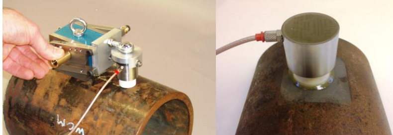
Left: The installation tool for straight pipes (Mag-ST) and a Wi-Corr Bond ultrasonic sensor bonded to a straight pipe section.
